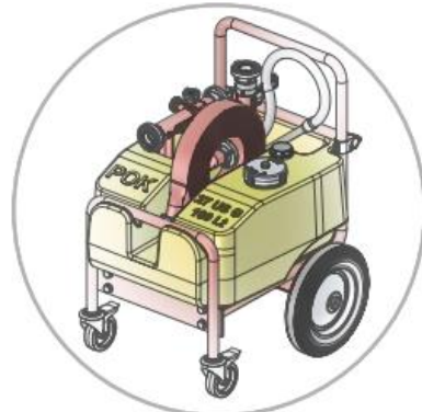
Mobile foam unit with 100 liters tank, "MIXY EDUCTOR" 200 lpm and low expansion foam nozzle 200 lpm
